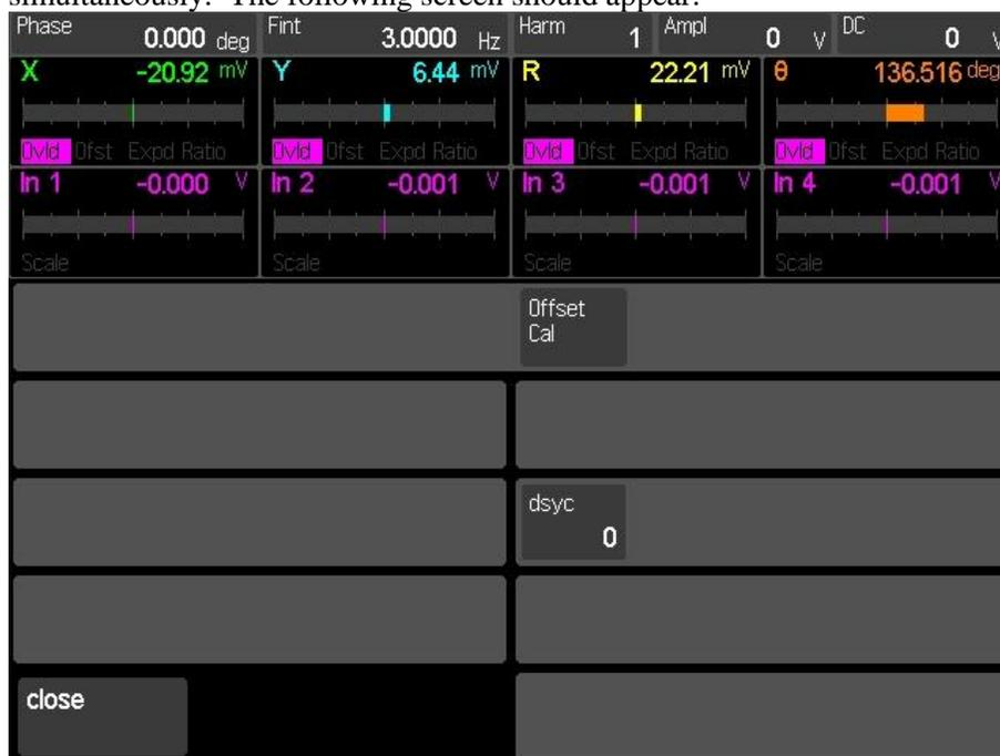
23. The “Offset Cal” tile will perform a single offset voltage. “Offset Cal” must be performed for each of the 5 input range settings (10 mV through 1 V), and for AC and DC coupling separately. Each calibration will require **about 1 minute** to complete, for a total of 10 minutes.
